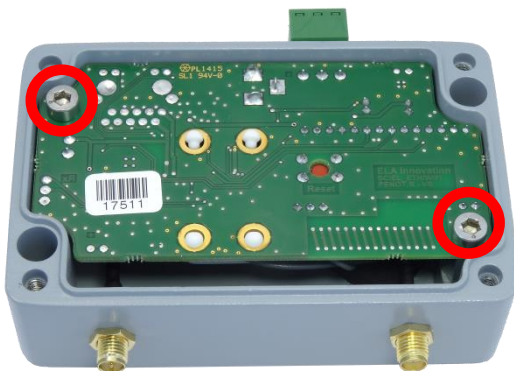
Image 9: Main board's screws
